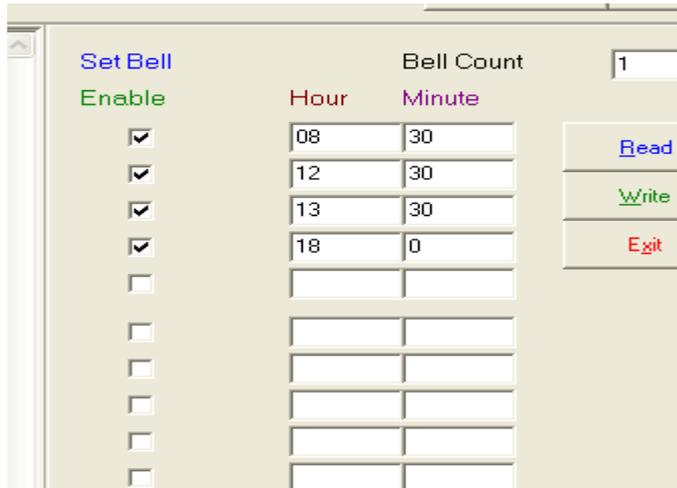
When you finish the input, you can press the button “write” to set the time to the device. Also, you can click the button “read” to read back the current bell time of the device.
