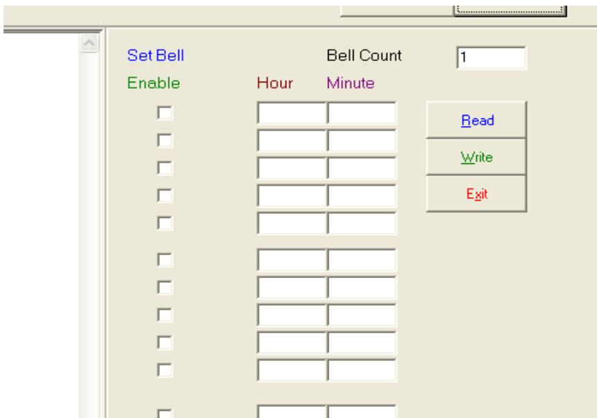
In the setting of bell time, you can input the hour and minute for the bell of the device to sound. When you start to input the hour, the “enable” check box will be checked automatically.
