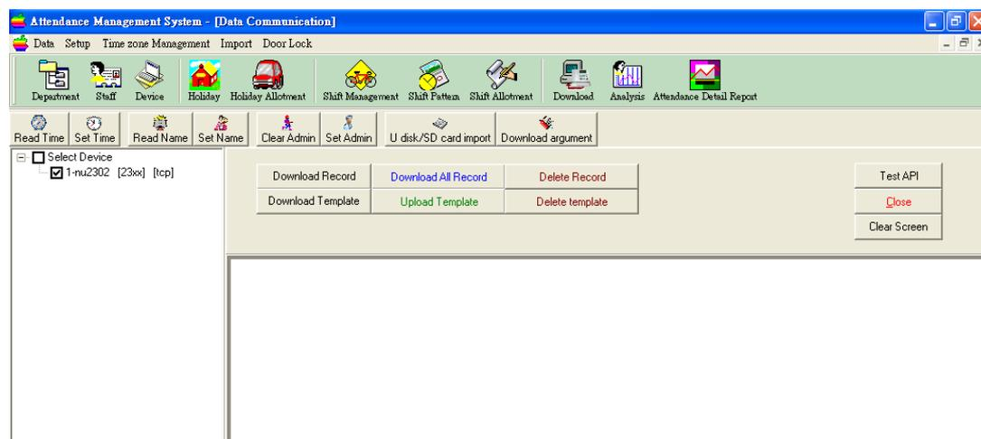
In the left side, you can see a tree list of devices that you input in Device Management. Each item has a square box in left hand side. Click the square box means you want to communicate with the device.
